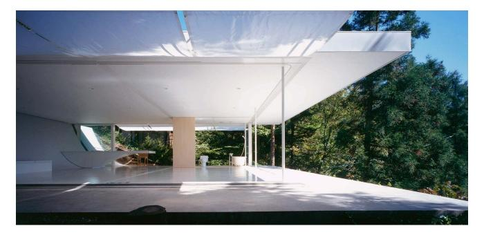
The Wall-less House sits on a mountain slope with the floor sloping upward to meet the roof, naturally absorbing the imposing load of the earth. The flat roof is fixed rigidly to the upturned slab, freeing the three front columns from taking any lateral loads achieving incredibly slender columns. The different functions of the house are placed without enclosure on an universal floor, further emphasizing the structural system, but can be partitioned off by sliding walls.
